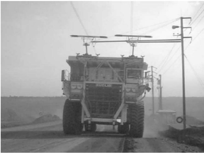
Fig. 6. Haul truck operating with trolley lines.
