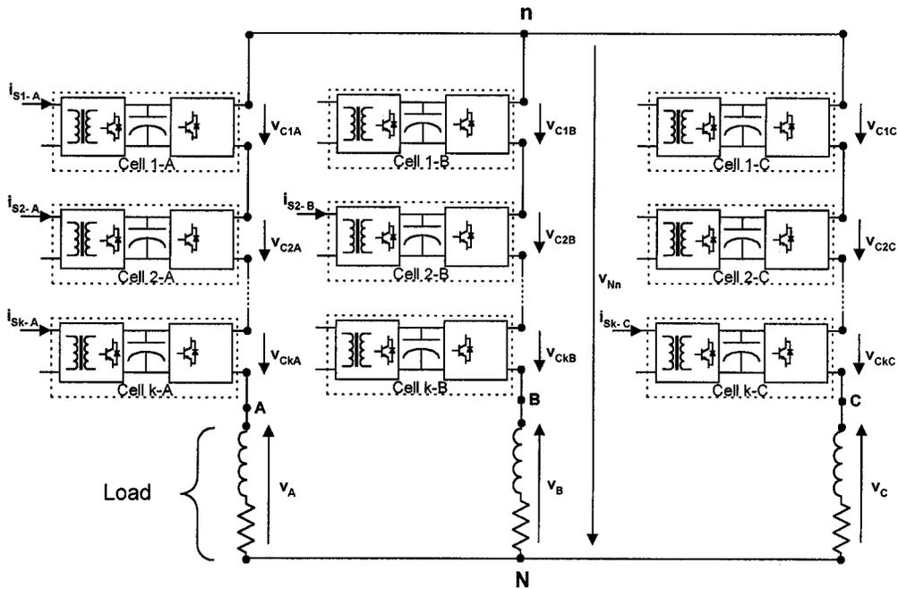
Fig. 2. Power circuit of the multilevel regenerative converter.
