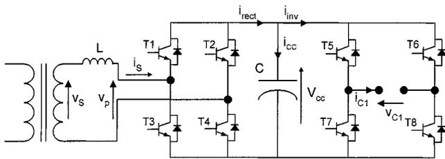
Fig. 3. Power circuit of the regenerative cell.
