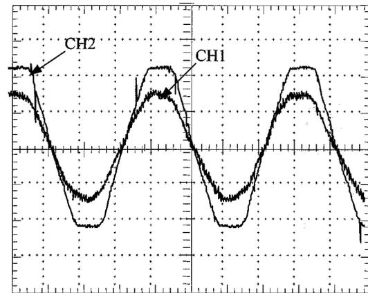
Fig. 18. Motoring mode waveforms of  $i_s$  (CH1 5 A/div) and  $v_s$  (CH2 25 V/div).
