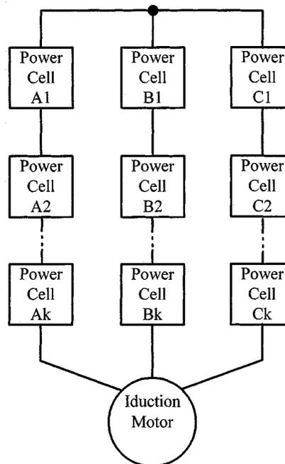
Fig. 1. Power circuit of a multicell inverter.
