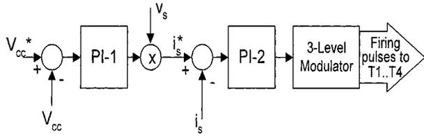
Fig. 6. Control system of the PWM rectifier.
