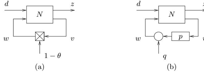
Fig. 2. System  $N$  with feedback over (a) erasure channel with dropout probability  $1 - p$ , and (b) additive noise channel with gain  $p$ .
