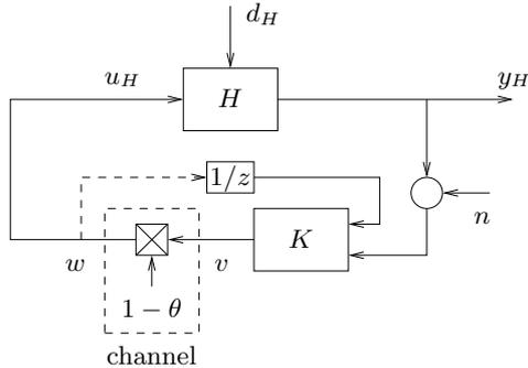
Fig. 4. SISO plant controlled over an unreliable channel.
