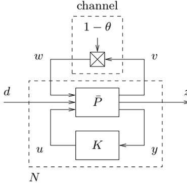
Fig. 1. LTI control system closed over a scalar erasure channel.
